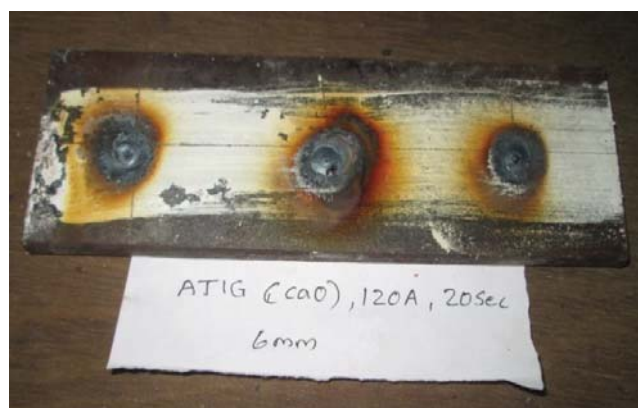
Fig 5. ATIG Spot welded specimen.
