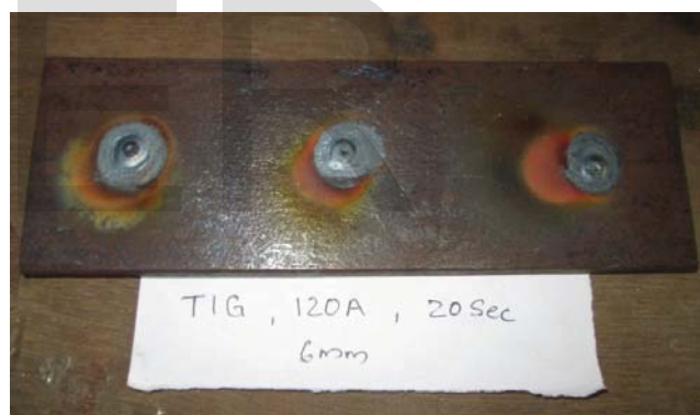
Fig 4. TIG Spot welded specimen.
